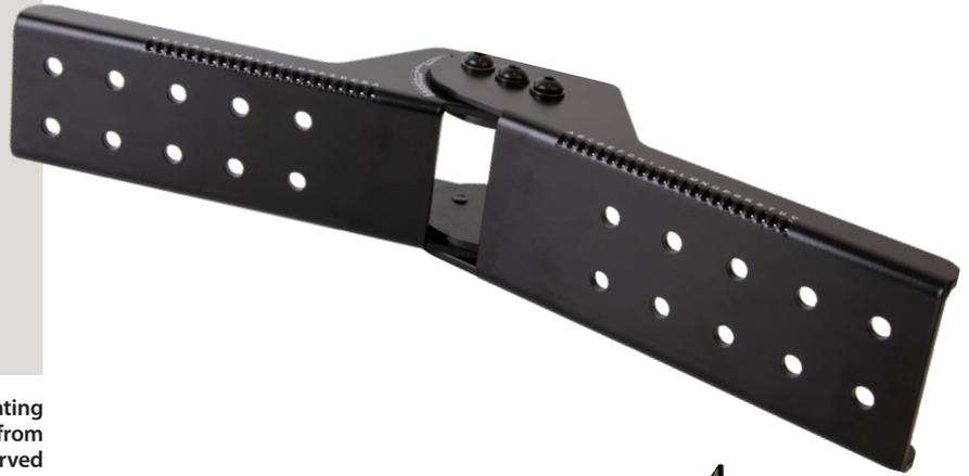
The BT8390-AAC is a connector that allows System X mounting rails to be joined together with an adjustable angle from -45° to +45°. This enables a solid, stable installation of curved multi-screen displays such as videowalls and menu boards and facilitates an installation process which is both quick and simple, aided by integrated angle guides.
