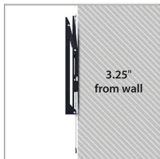
Mounts screen just 3.25" from the wall when mounted flat
