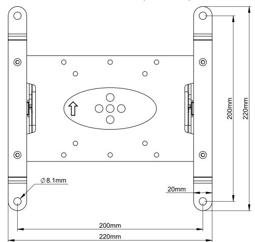
Revision: R00 UNLESS Size: A3 OTHERWISE SPECIFIED Scale: **Date:** 4/13/2021 See views **DIMENSIONS ARE** IN MILLIMETERS Sheet: 2 of 2 File Name: BTD-BT8420
